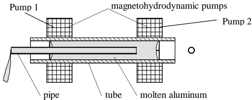
Plating steel pipes
