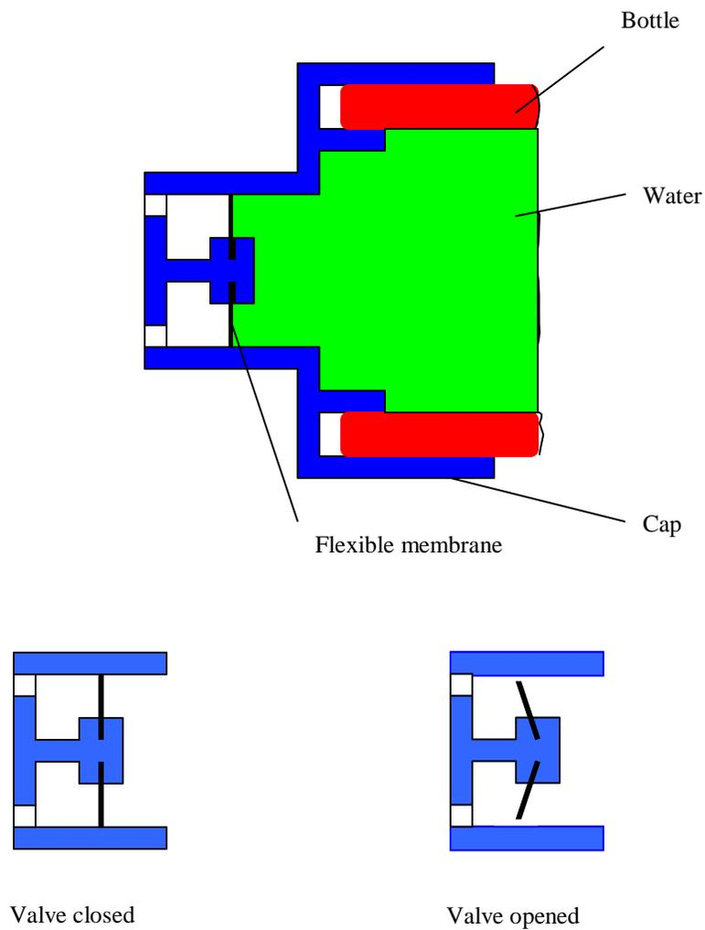
Water bottle cap with a flexible membrane
